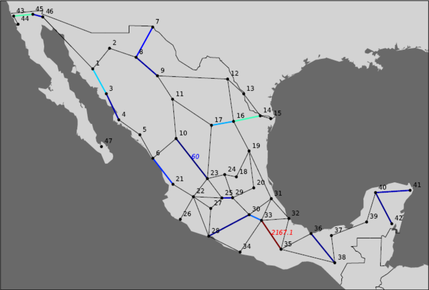
Minimum Transmission Capacity Added (MW) Mexico 2050
