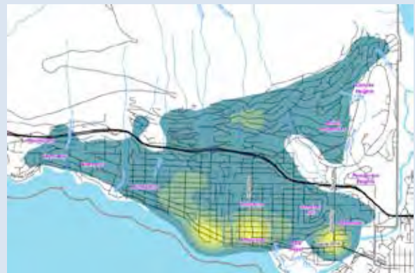
Figure 10: Thermal density analysis identifies area with high concentrations of space heating and hot water demand. Thermal density is amongst the most important factors in screening for district energy potential. Mapping: Golder and Associates for District of West Vancouver (Boston, 2015)
